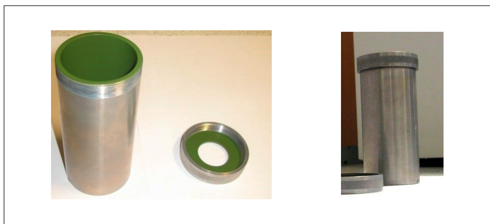
FIGURE 9/5: (05/18) Sample Can and Lid (both with threads)
