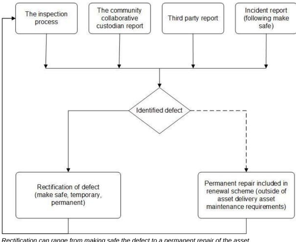
Figure E/1.15.1 Repair identification workflow
