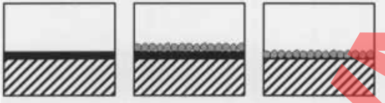
Figure 8.1 Single surface dressing
