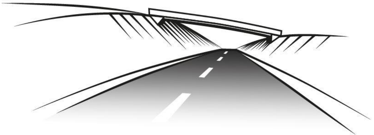
Figure 3.8 Illustration of maximum use of local topography to minimise the need for stairs and ramps
