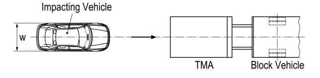
Figure 2.11b Head-on centre, 1/3 vehicle width offset
