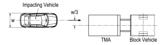
Figure 2.11c Nose 1/4 vehicle width offset, at 10 degrees
