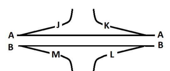
Figure E/1.7 Carriageway identifiers on connector roads
