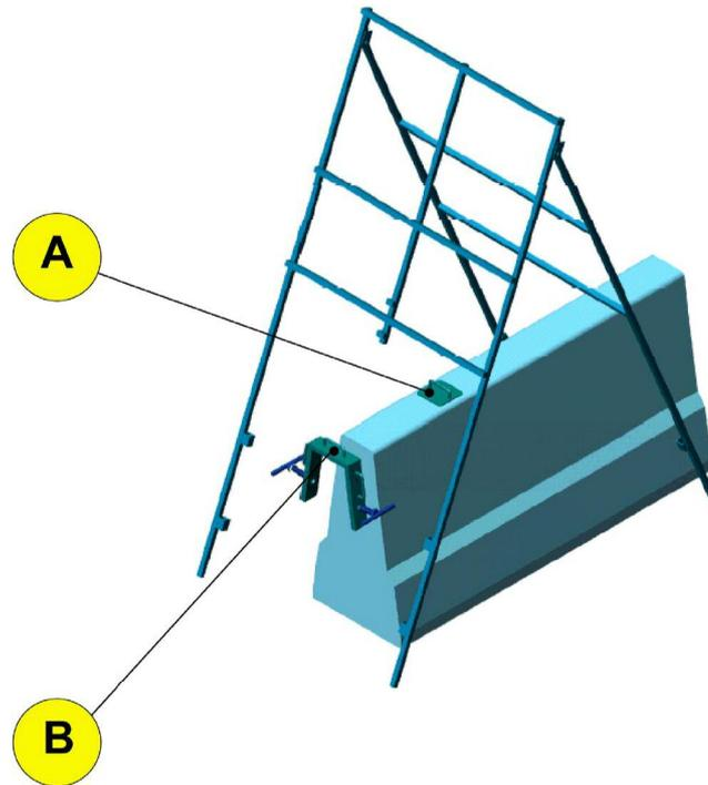
**Figure 6: Location of 'A' frame securing brackets on a concrete safety barrier**
