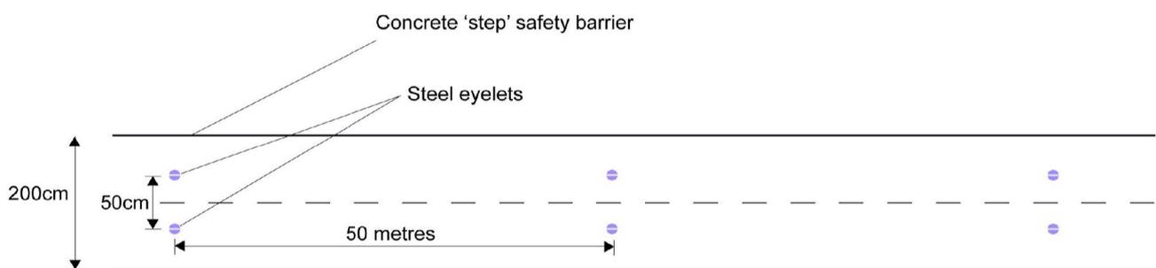
**Figure 9: Steel eyelets installed on the top surface of concrete safety barrier (plan view)**
