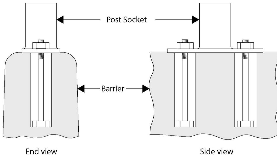
**Figure 7: Schematic of a type of retro-fit square post sign mounting in use in the United States**
