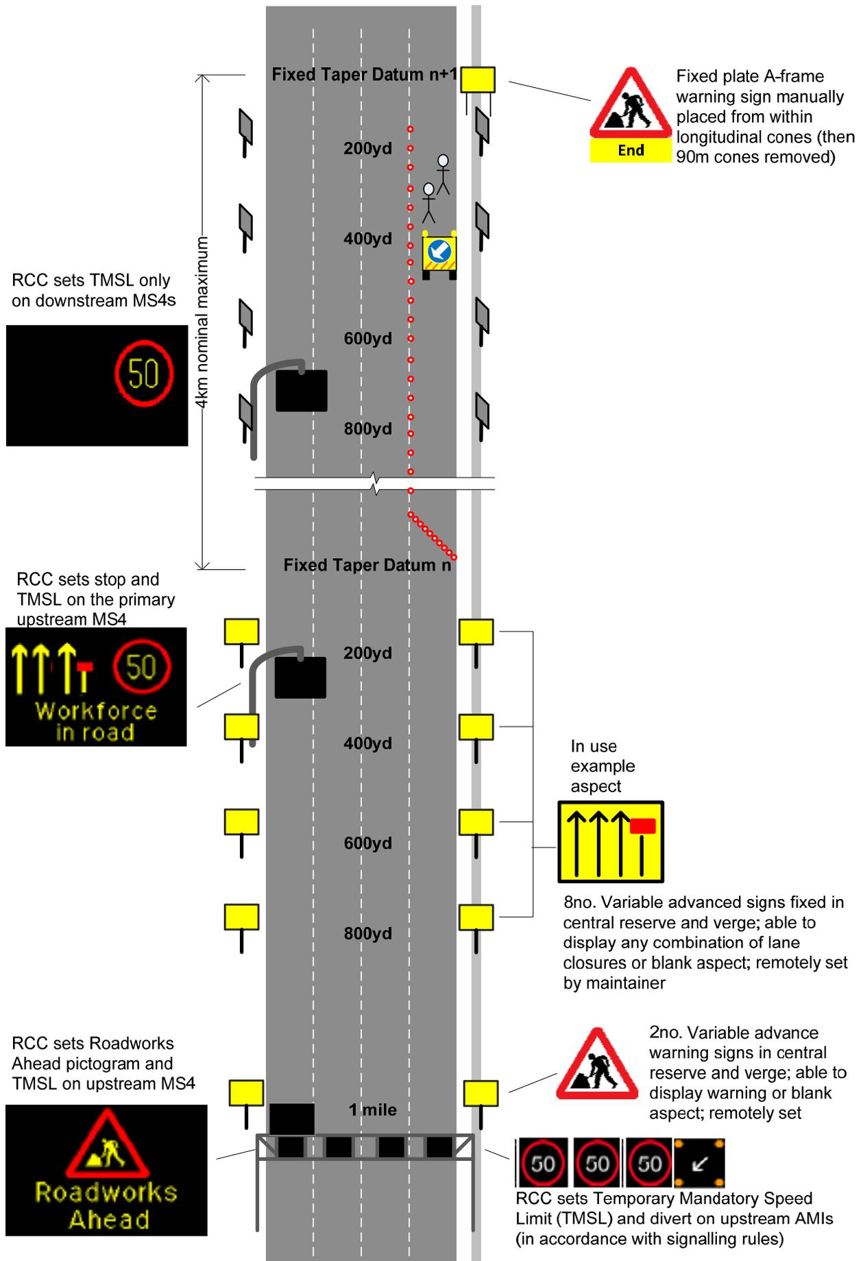
Figure 3: Works in progress in Lane 4 400yd upstream of FTP datum n+1. Note that aspects depicted on electronic scheme signals are indicative only.
